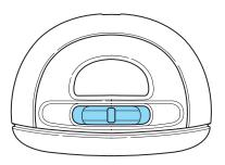
With the switch in the on position, the lamp will stay on all the time. In the off position, the lamp will stay off even when the doors are opened. With the switch in the center position, the lamp will turn on when the doors are opened and the top of the panel dimmer control is pressed to the full on position.
